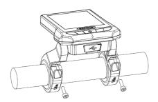
Open the clamp on the control pad and place it in the correct position, Using 1 X M3\*8 screw tighten the control pad onto the handlebar. Torque requirement: 1N.m.
