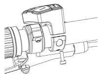
Please link the cable of control pad (B) to the display unit and link the display unit (A) to the EB-BUS cable.
